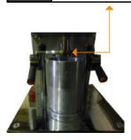
Turn the blocking lever so that the mould is secured to the base.
